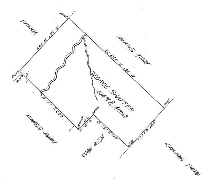
Draught of a tract of land Called\_\_\_\_ Situate on the waters of of Nescopeck Creek about three ·Miles from the N.E. Branch of Susqueha Joining Land Survey for Jacob Shatter of others in Catawassey Township Northumba County Containing four Hundred & four Acres & alloward of Six P Cent for Roads &c. Surveyed for George Shaffer the 10#66) of April 1787 in Pursuance of a Warrant Dated the 12th Day of Feb & 1786.
